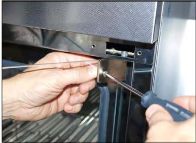
5. Turn the fitting slightly to the side, so that you can pull the hinge pin from the appliance. If the fitting is jammed due to heat exposure, carefully loosen it with a flat-head screwdriver.
