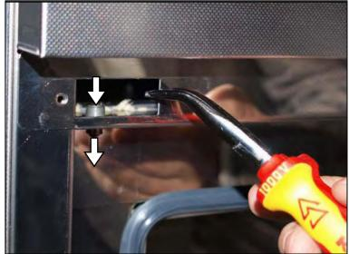
9. On the right side, insert the spring pressure pieces into the sleeves on the top and bottom.
